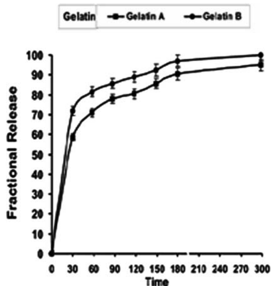
Fig. 11. Effect of type of gelatin on the released amount of insulin for a definite composition of nanoparticles [gelatin] = 2.0 g, [glutaraldehyde] = 10.6 mM, pH = 7.4, % loading = 49.7%.
